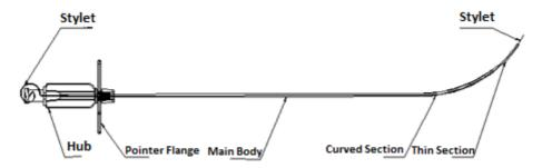
Pathbuilder<sup>™</sup> Transseptal Needle is consisted of thin section, curved section, main body, pointer flange, hub and stylet. The pointer flange indicates the curve orientation of the Pathbuilder<sup>™</sup> Transseptal Needle. The thin section of the Pathbuilder<sup>™</sup> Transseptal Needle fits well with that of the dilator which fixes the maximum length of the needle into the dilator.
